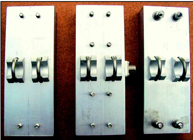
Figure 3—A top view of the antenna mounting plates.
